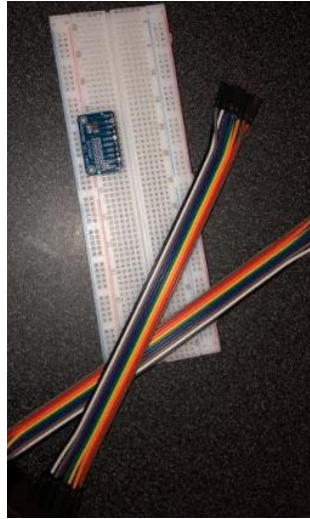
Figure 14: 16-Bit A/D, Breadboard, Jumper Cables
